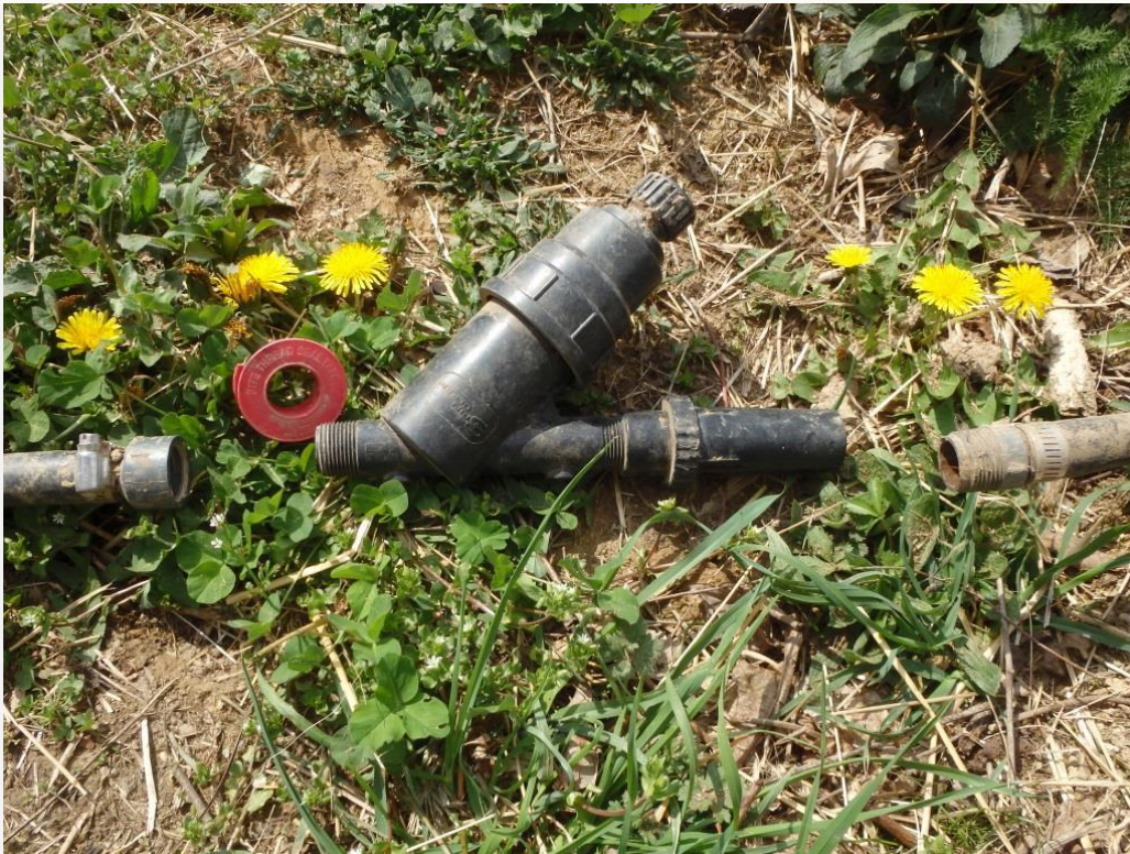
Header line with Female Adapter, Filter, Pressure Regulator, and Male Adapter
